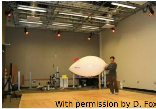
Fig. 3.8 Combination of a parametric prior and GPs for modeling and learning to control an autonomous blimp [34].
